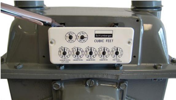
3. Remove the old gasket and any gasket residue from the meter and the index cover.
