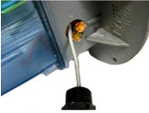
8. Replace the strain relief and tighten until secure.
