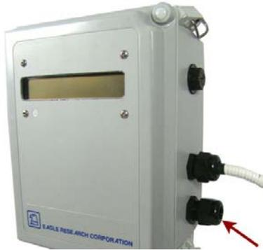
8. Pull the lead wires through the compression connector until there is adequate wire to reach the K2 terminal port.
