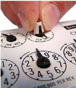
6. Press the magnet hub spacer down over the dial needle as far as possible. The tip on the bottom of the spacer may touch index face. Turn the dial in the direction noted on the index after hub spacer installation to verify the index dial functions with a smooth, easy rotation.
