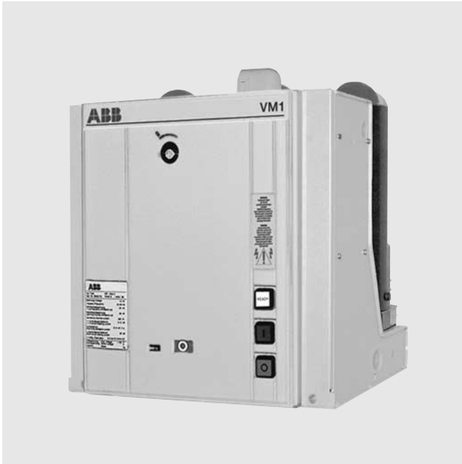
Figure 9/1: Vacuum circuit-breaker, type VM1, for fixed installation, 12 kV, \leq 1250 A, \leq 31.5 kA, mechanism side.
