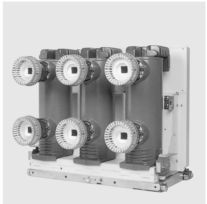
Bild 9/8: Vacuum circuit-breaker type VM1, high current, on withdrawable part, 12 kV, 3150 A, \leq 50 kA, pole side.
