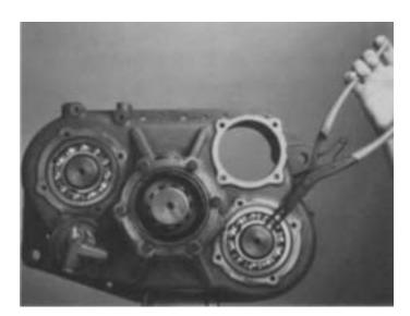
2. Remove the snap ring from groove at rear of each countershaft.
