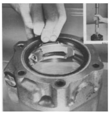
**16.** If previously removed, install the oil seal in rear bearing cover (inset). Seal should be installed so the spring is to the front of cover.
