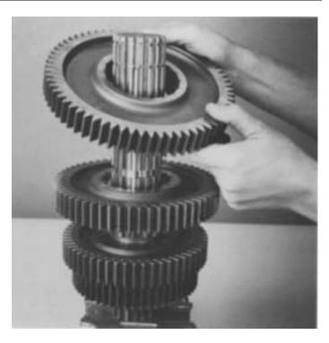
**14.** Install the 1st speed gear on shaft against 2nd speed gear, clutching teeth up.
