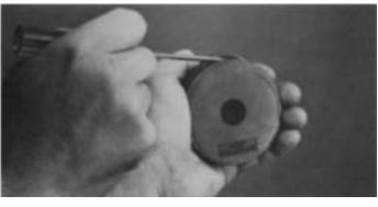
5. If previously removed, install the O-rings in the I.D. and O.D. of range piston.
