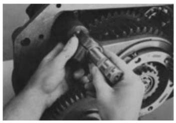
3. Place the range yoke into position with sliding clutch of synchronizer assembly, long hub of yoke to the rear. Insert threaded-end of yoke bar through yoke and into bore of range cylinder housing, aligning the notches in bar with yoke lockscrew holes.
