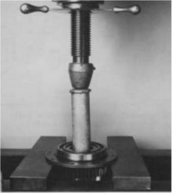
**5.** Using the rear face of retainer ring as a base, press the drive gear through bearing.
