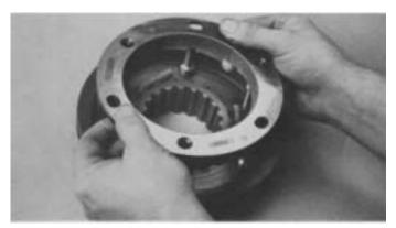
2. Place the larger low range synchronizer ring on bench and pull the high range synchronizer from blocker pins. However, before doing so, cover the assembly with a shop rag to prevent losing the three springs released from high range synchronizer at pin locations.
