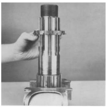
5. Remove the splined spacer from output shaft.
