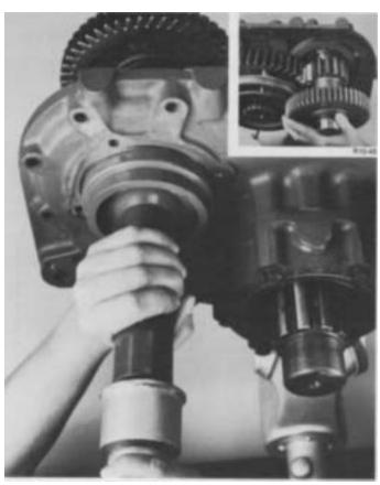
3. Place one of the assemblies into position in rear plate, meshing the marked tooth of countershaft low range gear with either set of two marked teeth of low range gear on output shaft (inset). Center rear of countershaft in bearing bore, start rear bearing in bore and complete installation with a flanged-end driver and maul. Repeat the procedure with other auxiliary countershaft assembly, making sure the low range gear set remains in time during bearing installation.
