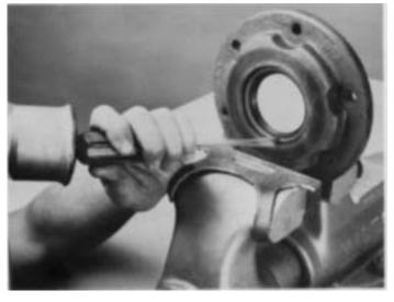
2. If necessary remove the oil seal from cover of models so equipped.
