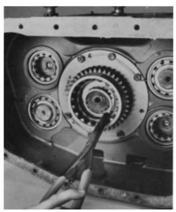
1. Remove the snap ring from groove at rear of mainshaft.
