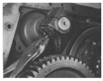
**4.** Install the two yoke lockscrews, tighten and wire securely.
