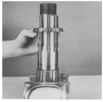
2. For 14610 models, install the spacer with large diameter spliNes down.
