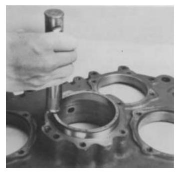
8. Install the front bearing cup in bore of auxiliary plate, taper to the inside. Use a soft bar to start cup into bore.
