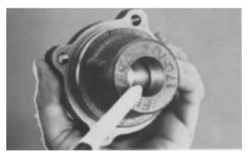
Remove the deep reduction cylinder housing and gasket from auxiliary housing. If necessary, remove the small O-ring from bore in cylinder housing.
