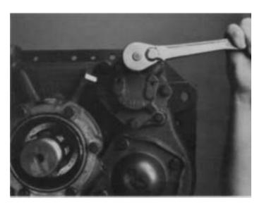
7. Position the corresponding new gasket on cover mounting surface and install the range cylinder cover on housing, open port to the upper left. Tighten capscrews to secure cover to housing.
