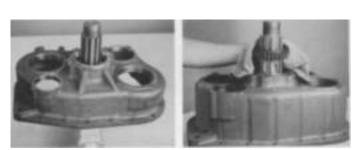
**12.** If not previously done so, install the auxiliary housing over end of output shaft assembly. Heat the rear bearing cone and install on shaft, taper down and inside bearing cup.
