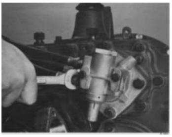
1. Disconnect and remove the 1/4" I.D. air line between the slave valve and air filter/regulator assembly.
