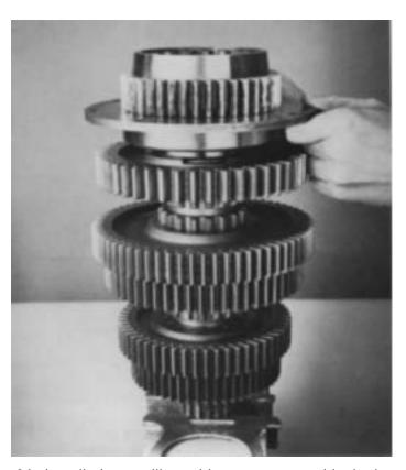
**24.** Install the auxiliary drive gear assembly in its proper position on rear of mainshaft.
