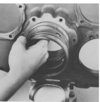
**6.** Remove the two bearing cups and outer spacer from bore in auxiliary housing.
