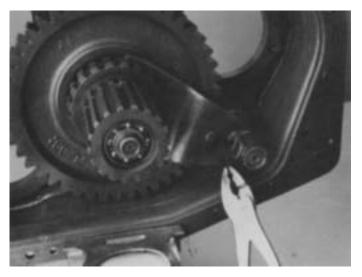
Install the yoke lockscrew, tighten and wire securely.
