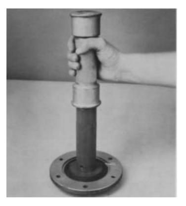
4. If previously removed, install the oil seal in drive gear bearing cover of models so equipped.
