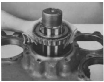
11. Install the auxiliary plate over end of output shaft assembly. Heat the rear bearing cone and install on shaft, taper down and inside bearing cup. NOTE: DO NOT HEAT BEARING ABOVE 275°F (136°C).
