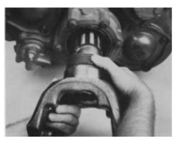
For models so equipped, install the speedometer drive gear or replacement spacer in position on hub of companion flange or yoke. Install the companion flange or yoke on splines of output shaft and move into rear bearing cover.
