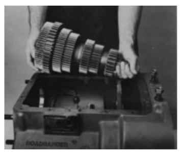
**2.** Place the right countershaft assembly into position in case, making sure that the "R"-marked assembly has the smaller 45-tooth PTO gear.
