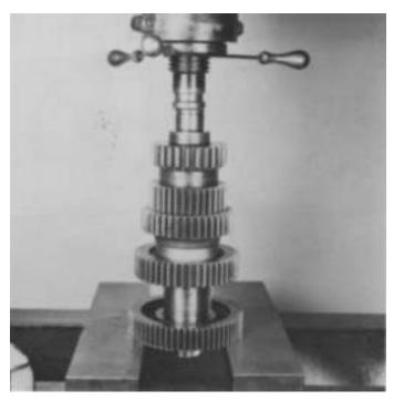
**4.** Press the 4th speed (or Overdrive) gear on countershaft, long hub of gear to the front of shaft.
