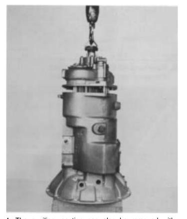
4. The auxiliary section can also be removed with transmission set in the vertical position. Block under the clutch housing to prevent damage to the input shaft, remove the retaining capscrews in housing flange and lift the assembly from front section. Remove gasket.
