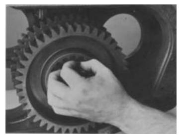
**4.** Install the key in keyway of range mainshaft, inserting the thick end of key in square internal spline of tolerance washer to lock low range gear on shaft.
