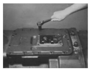
**3.** Install the capscrews in housing and tighten to secure the assembly to case.
