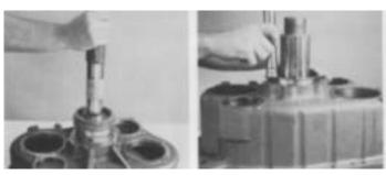
11. Stack the bearing outer spacer and rear bearing cup on top of the front bearing cup in proper sequence. Use a soft bar or a flanged driver to move all three parts evenly into housing bore until lip of rear bearing cup seats on housing.
