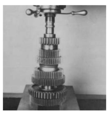
5. Start the PTO gear onto countershaft, bullet-nose side of teeth facing up and toward rear of shaft. Align keyway of drive gear with key in countershaft and press BOTH gears onto shaft, long hub of drive gear against PTO gear.
