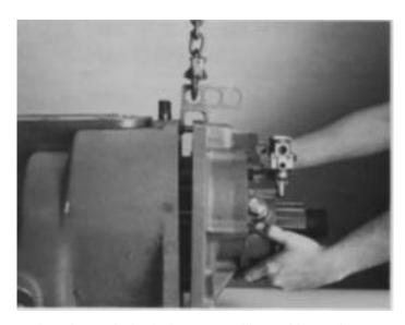
Attach a chain hoist to auxiliary. Move the assembly evenly into rear of front case, piloting it on the dowel pins. As assembly is moved forward, the countershaft drive gears will mesh with the auxiliary drive gear. IMPORTANT: On 15-speed auxiliary sections,
