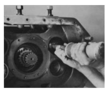
**5.** From the rear of case, use a soft bar and maul to drive each countershaft forward to unseat the front bearings from case bores and expose the bearing snap rings.
