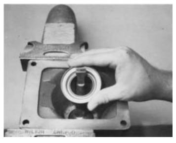
2. Position the gear shift lever in housing with spade pin in leaver ball slot and install the tension spring washer over ball, dished-side up.
