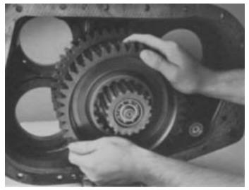
2. Install the low range gear on mainshaft against couplete, clutching teeth.
