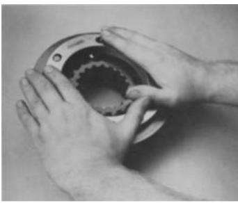
4. Apply downward pressure to the high range synchronizer ring WHILE TWISTING COUNTER-CLOCKWISE to compress the springs and fully seat ring on blocker pins of low range synchronizer.
