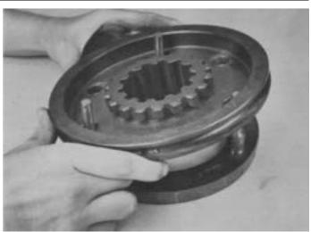
**3.** Remove the sliding clutch from pins of low range synchronizer ring.
