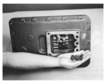
2. Tilt the assembly and remove the three sets of tension springs and balls from the housing bores.
