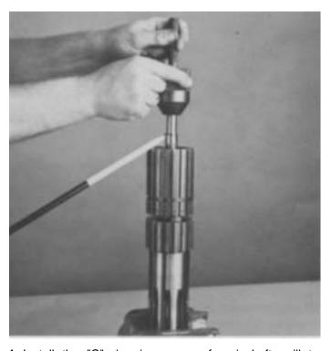
**4.** Install the "C" ring in groove of mainshaft quill to retain bearing.
