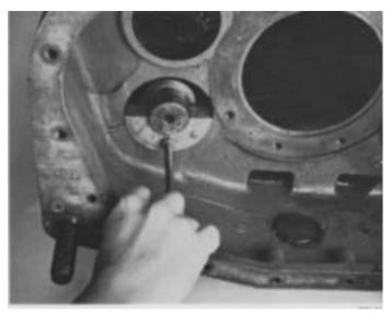
1. Move the left countershaft assembly to the rear and insert countershaft support tool or blocking to center shaft in rear case bore.
