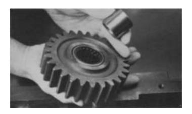
7. If necessary, remove the inner race from bearing and press needle bearing from idler gear.
