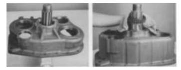
13. For models equipped with the oil retention ring in auxiliary housing, install the speedometer drive gear or replacement spacer on output shaft and retain with snap ring installed in groove of shaft (left). Remove the blocking (two mainshaft spacers or flat steel stock) from between the deep reduction gear and auxiliary housing (right).
