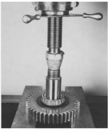
3. Using the front face of low range gear as a base, press the output shaft through the gear and bearing. Remove the bearing and washer from hub of low range gear.
