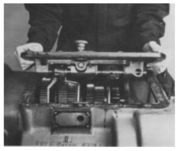
Install the new shift bar housing gasket in position on case.
