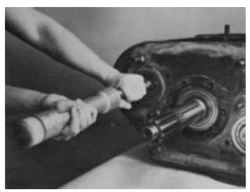
4. Use a soft bar and maul to drive each countershaft to the rear as far as possible. This will partially unseat the front bearings.
