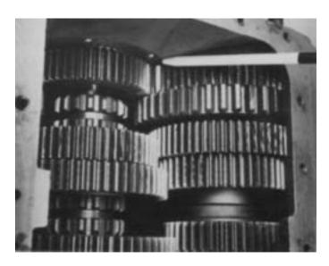
Remove blocking from right countershaft assembly and place it parallel to mainshaft assembly. Mesh the marked tooth of right countershaft drive gear with remaining set of two marked teeth on main drive gear.
