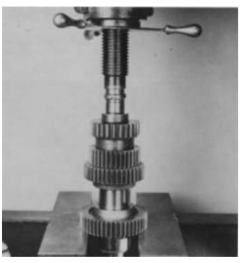
**3.** Press the 3rd speed gear on countershaft, long hub of gear against 2nd speed gear hub.
