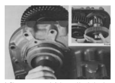
3. Place one countershaft into position in housing, meshing the marked tooth of countershaft gear with either set of two marked teeth of mainshaft deep reduction gear (inset). Center rear of countershaft in bearing bore, start rear bearing in bore and complete installation with a flanged-end driver and maul. Repeat the procedure with other auxiliary countershaft assembly, making sure the deep reduction gear set remains in time during bearing installation.
