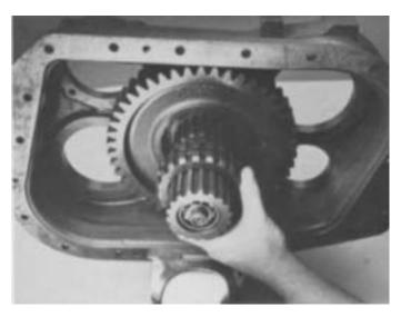
2. Remove deep reduction sliding clutch.
