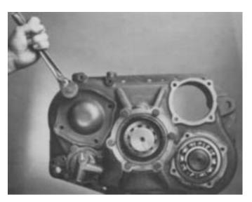
Turn out the capscrews and remove both countershaft rear bearing covers.
