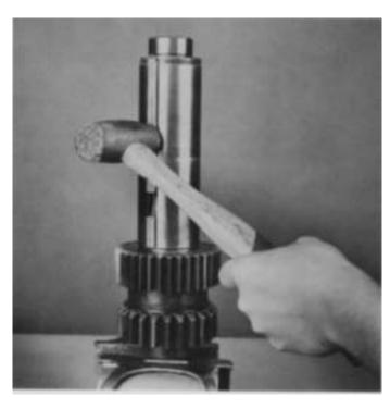
**1.** If previously removed, install the roll pin and key in keyway of countershaft.
