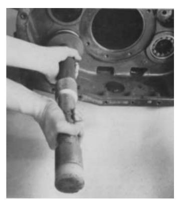
**6.** Remove countershaft support tool or blocking from rear case bore and install the left countershaft rear bearing with larger I.D. lead chamfer to the front of shaft and install the snap ring in groove at rear of left countershaft.
