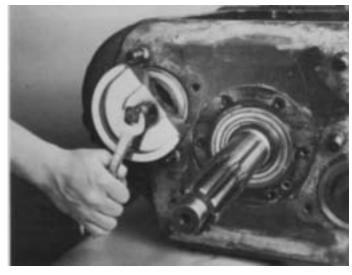
**6.** Use a bearing puller or pry bars to remove the countershaft front bearings.
