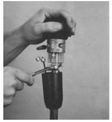
Loosen the jam nut and turn the Roadranger Valve and nut from gear shift lever. Remove the valve cover, air lines, sheathing and O-rings from lever.
