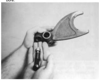
**8.** If necessary, remove the plug, spring, and reversestop plunger from the LO-Reverse speed shift yoke bore. B. Reassembly of the Shift Bar Housing Assembly.
