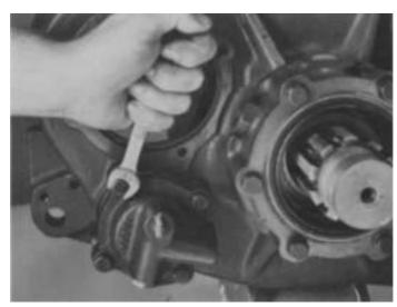
**6.** Position the corresponding new gasket on cover mounting surface and install the deep reduction cylinder cover, aligning the air channel with channel in cylinder housing. Tighten capscrews to secure cover to cylinder housing.
