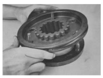
1. Place the larger low range synchronizer ring on bench and install the sliding clutch on blocker pins, recessed side up.
