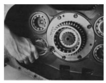
**2.** Cut lockwire and remove the capscrews from bearing retainer ring.
