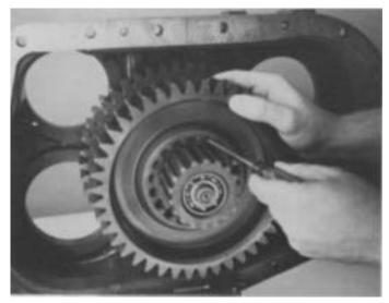
2. Turn the washer located in the hub of low range gear so that the splines of washer align with the splnes of mainshaft.
