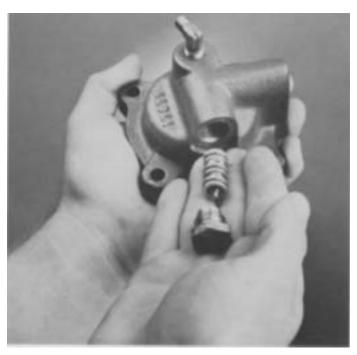
2. If necessary, turn out the insert valve retaining nut of covers so equipped and remove insert valve from bore.
