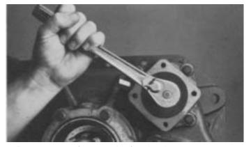
2. Remove nut from end of yoke bar.
