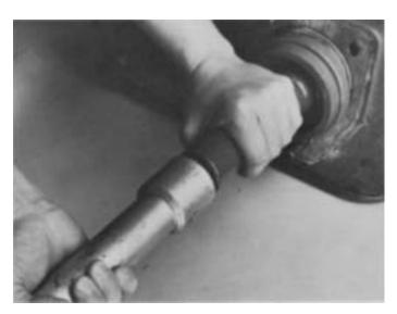
**4.** Use a flanged-end bearing driver to completely seat front bearing or bearing outer race in case bore.
