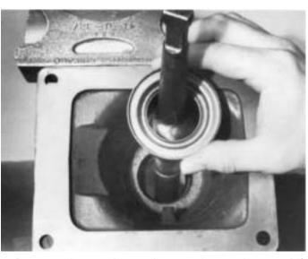
**3.** Remove the tension spring, washer and gear shift lever from housing.
