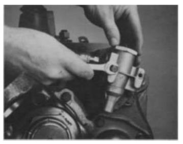
3. Turn out the two capscrews and remove the air filter/regulator assembly.
