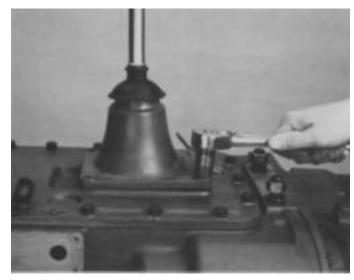
**3.** Install the retaining capscrews in housing flange and tighten to secure the assembly to shift bar housing.
