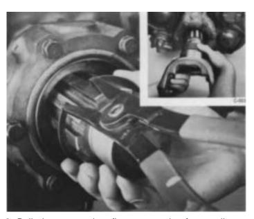
2. Pull the companion flange or yoke from splines of output shaft. Remove the speedometer drive gear or replacement spacer from hub of flange/ yoke or from inside rear bearing cover remaining on output shaft (inset). For some models, it is necessary to remove the snap ring in groove of output shaft PRIOR to removal of the speedometer gear or spacer.
