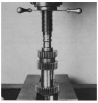
2. Align keyway of gear with key in countershaft and press the 2nd speed gear on shaft, long hub of gear to the front of countershaft.
