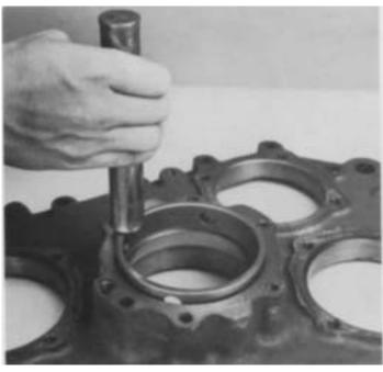
**9.** Place the bearing outer spacer against cup and use a soft bar or flanged-end driver to move both parts evenly into bore.
