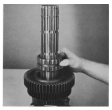
**10.** Install the 2nd-3rd speed sliding clutch, aligning the missing internal spline of sliding clutch with key in mainshaft.
