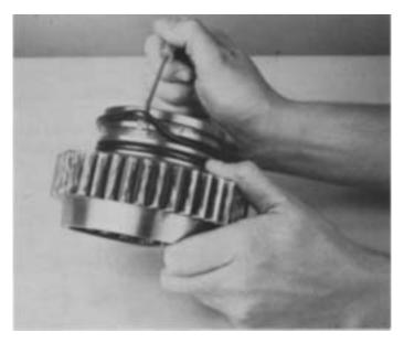
**6.** If necessary, remove the O-rings from hub O.D. of auxiliary drive gear.
