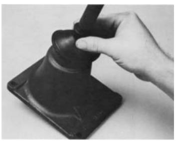
**4.** Remove the assembly from vise and install the rubber boot over gear shift lever and against housing.
