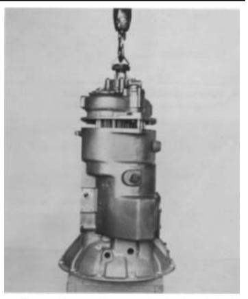
3. The auxiliary section can also be installed with transmission set in the vertical position. Block under the clutch housing to prevent damage to the input shaft, position the corresponding new gasket on plate/housing mounting surface and lower the assembly onto rear of front case. Install the retaining capscrews and tighten securely. See TORQUE RECOMMENDATIONS,
