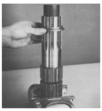
1. Remount the output shaft in vise with threaded-end up and secure on range mainshaft. For models so equipped, install the stepped washer on shaft, large diameter step down.
