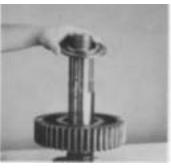
5. Install the washer on shaft against deep reduction gear, small diameter step down (Left: 11615 Models); or side with large groove up (Right: 15615 and 14615 Models).
