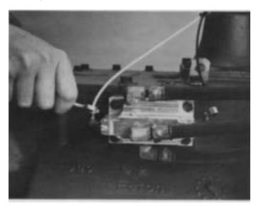
Disconnect the two I/8" O.D. air lines at the "S" or Supply Port and the "P" or End Port of slave valve on transmission case.
