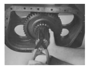
15. Install snap ring in groove of range mainshaft.
