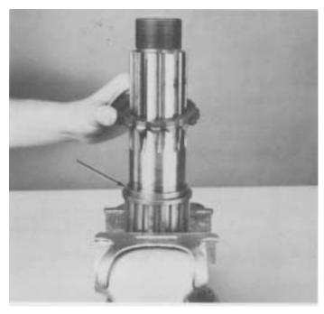
1. Secure the output shaft in a vise with threaded end up. For models so equipped, install the stepped washer on shaft large diameter step down (arrow), then install the splined spacer.
