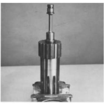
**1.** Secure the output shaft in a vise with mainshaft quill up.
