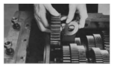
**6.** As the idler shaft and washer is moved to the rear, remove the thrust washer, and gear from case.
