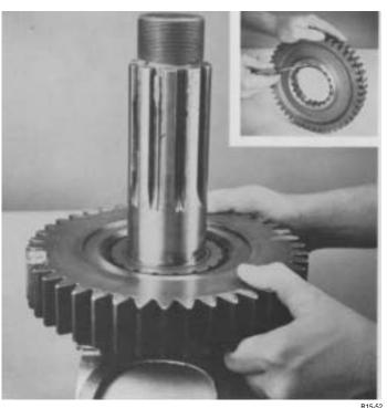
**4.** If previously removed, install the snap ring in deep reduction gear of models so equipped (inset). Install the gear on output shaft, clutching teeth down and engaged with splines of spacer.
