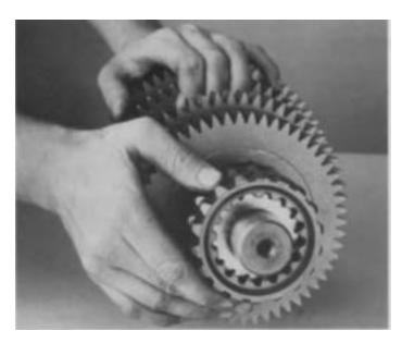
28. Remove the mainshaft assembly from vise. Align the missing internal spline of 4th-5th speed sliding clutch with key in mainshaft and install on front of shaft, engaging the external splines of sliding clutch with clutching teeth of 4th speed (or Overdrive) gear.
