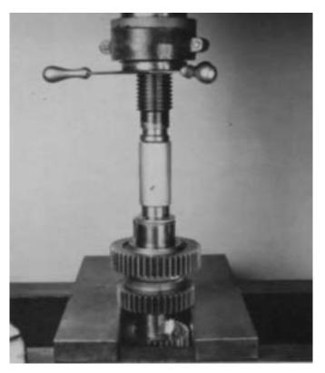
4. Using the rear face of 2nd speed gear as a base, press the 3rd speed and 2nd speed gears from each countershaft.
