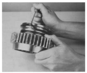
**1.** If previously removed, install the O-rings on extended front hub of auxiliary drive gear.
