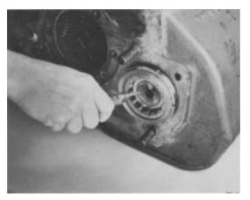
**3.** Center the front of left countershaft in bearing and move the assembly forward.
