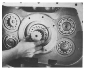
3. Align the external splines of spacer with clutching teeth of reverse gear and move spacer forward on mainshaft and into gear.
