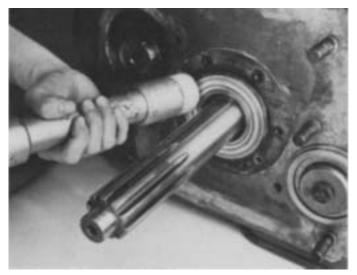
Tap the bearing into position in the bore with a soft mallet.
