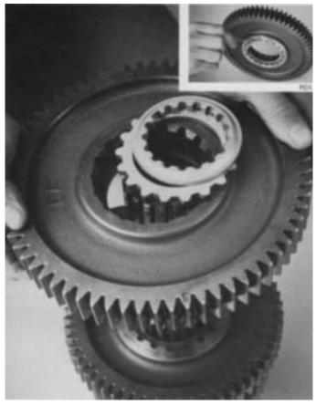
Pull the 1st speed gear from rear of mainshaft to remove limit washer, spacer and gear. If necessary, remove the snap ring from I.D. of gear (inset).
