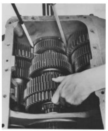
**31.** With the reverse gear remaining against 1st speed gear, mesh the corresponding forward speed gears of left countershaft assembly. Check to make sure that marked tooth on left countershaft drive gear has remained in mesh with marked set of teeth on main drive gear.
