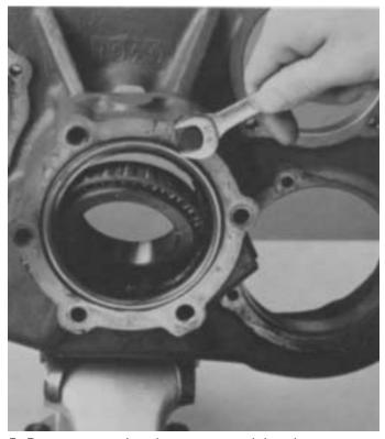
5. Remove rear bearing cover and bearing cone.
