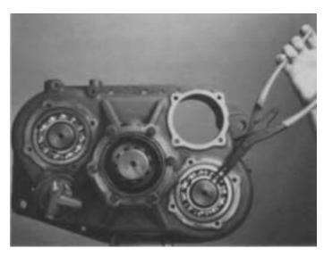
Install the snap ring in groove at rear of each countershaft.
