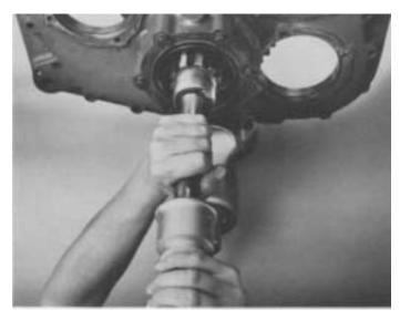
**1.** Use a soft bar and maul to drive the output shaft forward and through rear bearing assembly.
