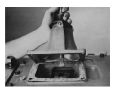
Install the new gear shift lever housing gasket in position on shift bar housing and install the gear shift lever housing assembly on shift bar housing, fitting the lever into shift block and yoke notches.
