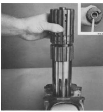
2. If necessary, press the bushing in rear bore of range mainshaft (inset) and install the mainshaft in position on quill.
