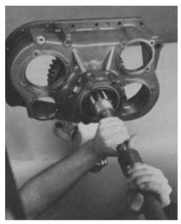
**4.** Use a soft bar and maul to drive the output shaft forward and through rear bearing assembly. This will cause the rear bearing cone to be released from bore in auxiliary housing.
