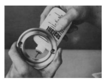
**1.** Apply Loctite grade 277 sealant to cleaned threads of new drive gear bearing nut. DO NOT REUSE OLD NUT.
