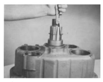
2. If not previously done so, remove the snap ring and speedometer drive gear or replacement spacer from output shaft of models so equipped.
