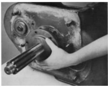
**1.** Turn out the retaining capscrews and remove the drivegear bearing cover and gasket.
