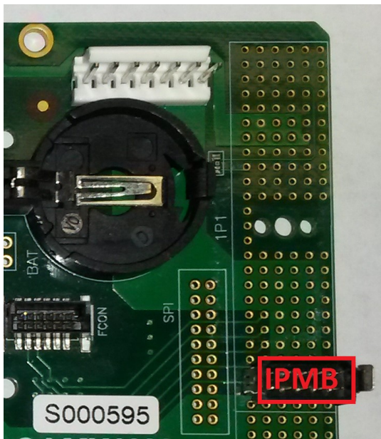
Figure 3 IPMB Connector Location
