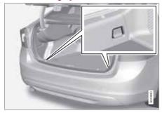
The folding load retaining eyelets are used to fasten straps in order to anchor items in the cargo area.
