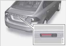
The boot lid is held closed by an electrically controlled lock. To open:
