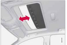
One long press on the lock button closes the sunroof and all the windows, see pages 43 and 54. The doors and the boot lid are locked. To interrupt closing, press the lock button again.
