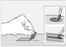
Before work is begun, the car must be clean and dry and at a temperature above 15  $^{\circ}$ C.
