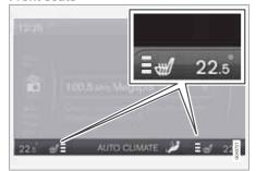
Current heat level is shown in the centre console display.
