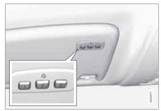
HomeLink® is a programmable remote control which can control up to three different devices (e.g. garage door, alarm system, outdoor lighting and indoor lighting etc.) and in doing so replace their remote controls. HomeLink® is supplied built into the left-hand sun visor.
