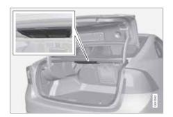
The backrest is in two sections, they can be folded forward, together or separately.
