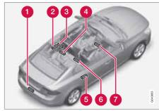
The keyless system has a number of integrated antennae located around the car:
