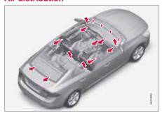
The incoming air is divided between 20 different vents in the passenger compartment.
