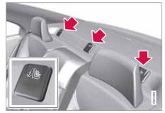
The car is equipped with upper mounting points for child seats. These mounting points are located on the parcel shelf and are con-
