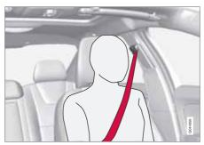
Correctly fitted seatbelt.
