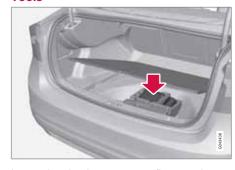
Located under the cargo area floor are the car's towing eye, jack\* and wheel wrench\*. There is also space for the sleeve for the lockable wheel bolts.
