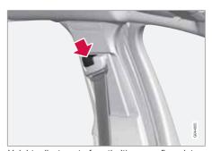
Height adjustment of seatbelt's upper fix-point. Press in the button and move the upper fix-point vertically. Position the upper fix-point as high as possible without the belt chafing against your throat.
