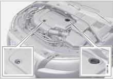
Dipstick<sup>1</sup> and filler pipe, diesel engine.
