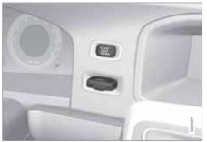
Ignition switch with inserted remote control key.
