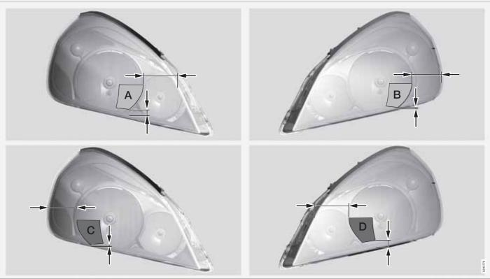
Upper row: masking left-hand drive cars, templates A and B. Lower row: masking right-hand drive cars, templates C and D.
