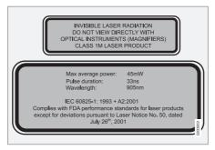
The upper label in the figure describes the laser beam's classification:
