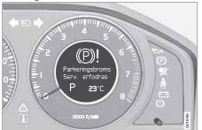
Park brake not fully released - A fault is preventing the parking brake from being released. Visit a workshop - an authorised Volvo workshop is recommended. A warning signal sounds if you pull away with this error message.
