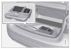
Emergency puncture repair (TMK; Temporary Mobility Kit) is used to seal a puncture and check and adjust tyre pressure. It consists of a compressor and a bottle with sealing fluid. The kit works as a temporary repair. The sealing fluid bottle must be replaced before its expiration date and after use.
