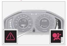
The warning symbol in the combined instrument panel illuminates when the remote control key is in key position II or III. The symbol clears after approx. 6 seconds provided the airbag system is fault-free.
