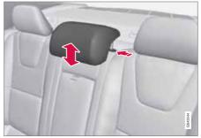
Adjust the head restraint according to passenger height so that the whole of the back of the head is covered if possible. Slide it up as required.
