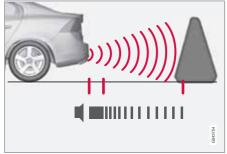
The distance covered to the rear of the car is about 1.5 metres. The acoustic signal for obstacles behind comes from one of the rear loudspeakers.
