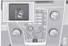
The function is switched on or off by means of a switch on the centre console. An indicator lamp in the button illuminates when the function is switched on.
