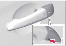
If central locking cannot be activated with the PCC, e.g. if the batteries are discharged, then the left-hand front door can be opened with the PCC's detachable key blade (see page 46).
