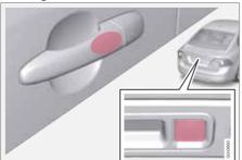
Cars with the Keyless system have a pressuresensitive area on the outer handle of the doors and a rubberised button next to the boot lid's rubberised pressure plate.
