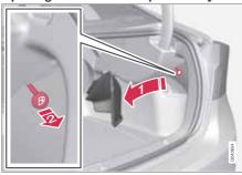
The fuel filler flap can be opened manually when electric opening from the passenger compartment is not possible.
