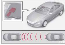
Laser sensor transmitter and receiver window.
