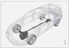
All Wheel Drive means that the car is driving all four wheels at the same time.
