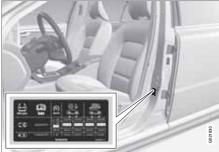
The tyre pressure decal on the driver's side door pillar (between frame and rear door) shows which pressures the tyres should have at different loads and speed conditions. This is also specified in the tyre pressure table, see page 333.
