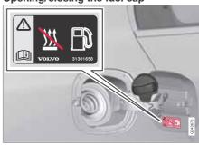
The fuel filler cap can be attached onto the flap.
