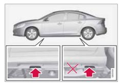
If the car is raised with a workshop jack; position the jack against the front edge on the engine's subframe.
