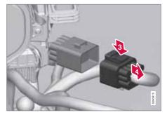
All of the headlamp bulbs are replaced via the engine compartment. Loosen and remove the whole headlamp.
