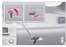
The glovebox can only be locked/unlocked using the remote control key's detachable key
