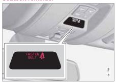
Unbelted occupants will be reminded to fasten their seatbelts by means of an audio and visual reminder. The audio reminder is speed dependent, and in some cases time dependent. The visual reminder is located in the roof console and the combined instrument panel.
