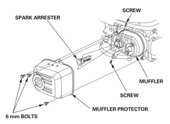
3. Use a brush to remove carbon deposits from the spark arrester screen.
