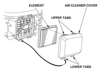
Remove the element. Carefully check the element for holes or tears and replace if damaged.
