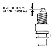
4. Check that the spark plug washer is in good condition and thread the spark plug in by hand to prevent cross-threading.
