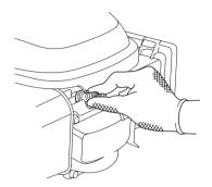
5. After the spark plug is seated, tighten with a spark plug wrench to compress the washer.
