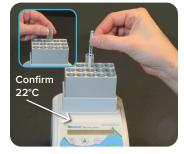
Place tube in Incubator and acclimate for 2 min.\*, then add QuickTox Strip; wait 5 minutes for results
