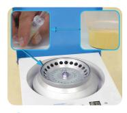
Centrifuge a portion of extract for 30 seconds at 2000 x q (NOT RPM).
