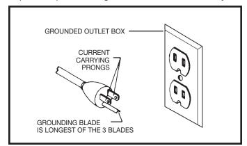
Repair or replace damaged or worn cord immediately.
