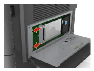
d. Tighten the two screws.
