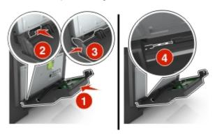
10. Run the ISP cable through the controller board shield.
