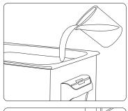
Fill the tank with warm or tap water below the maxline; Add required quantity of deaning solution. When using flammable liquid such as alcohol, gasoline and so on, heating is strictly forbidden! Ultrasonic vibration for a long time cause temperature of liquid increase, cau-tionfire.
