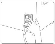
Plug the cleaner into a grounded oudet. Turn on the power switch at the ank back, then machine is power on.
