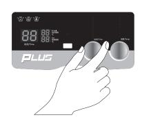
PLUS series: At first setting, the time is random, progress bar light on, turn the rotary knob clockwise to increase time. Turn counterclockwise to decrease time. Corre-spondinaly the two digits on the left of the display change accordingly, and the time setting done well. Press the rotary knob, ultrasonic start working.
