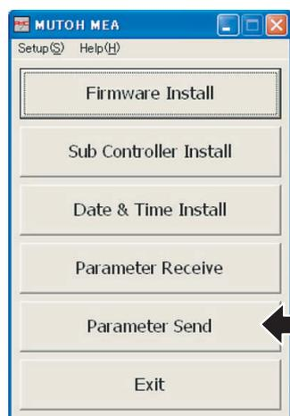
2. When the "Select of send parameter file" window opens, select the parameter file to be transferred and click [Open].
