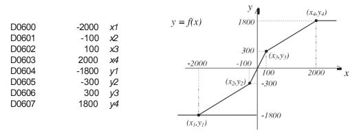
The FG instruction interpolators f(x) value for x based on the n parameters of  $(x_i, y_i)$ . For example, if XW04 is 1500 (x = 1500), the result 1405 (f(x) = 1405) is stored in D0100.
