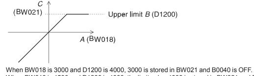
When BW018 is 4500 and D1200 is 4000, the limit value 4000 is stored in BW021 and B0040 is ON.
