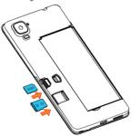
③ Ensure that SIM and microSD<sup>™</sup> cards have been properly secured.
