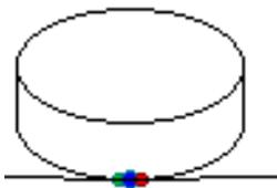
The wastewater is diverted to a large tank or holding pond that is used to provide a more uniform concentration of chemicals in the wastewater before biodegradation. The equalization unit is located before biological treatment. Agitators are sometimes used to promote mixing and cool the wastewater. High temperatures in biotreatment can cause reduction in the flocculation settling rates. The model for equalization is flexible and can model several types of equalization units.
