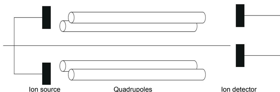
Figure F.2 Quadrupole Mass Spectrometer Diagram
