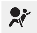
SRS warning light
