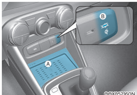
[A]: Charging pad, [B]: Indicator light
