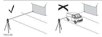
When measurements are being made using the red laser EDM, the results may be influenced by objects passing between the EDM and the intended target surface. This occurs because reflectorless measurements are made to the first surface returning sufficient energy to allow the measurement to take place. For example, if the intended target surface is the surface of a road, but a vehicle passes between the EDM and the target surface as **DIST** (F2) or **ALL** (F1) is pressed, the measure-
