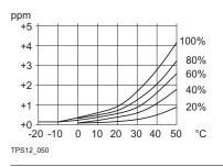
ppm % Air humidity correction [mm/km] Relative humidity [%] Air temperature [°C]
