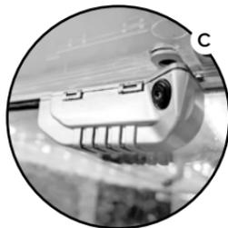
**!** Please make sure that the NTC sensor is not placed right against the substrate heating cable (blue cable) as it will give an inaccurate measurement.
