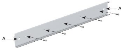
Figure 2: Drill cable entry (A) for connection cable in the mounting plate
