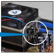
Align the other end of the retention bracket (near the retention bracket lock) to the retention module base. A clicking sound denotes that the retention bracket is in place.
