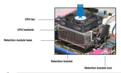
Your boxed CPU heatsink and fan assembly should come with installation instructions for the CPU, heatsink, and the retention mechanism. If the instructions in this section do not match the CPU documentation, follow the latter.
