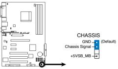
M2N/M2N DH Chassis Intrusion Connector
