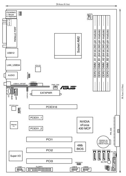
The USB910\_WFGBT module, and MP3-IN connector are available to M2N DH model only. The USB910 port is available to M2N model only. These items are greyed out in the given motherboard layout.
