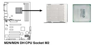
Unlock the socket by pressing the lever sideways, then lift it up to a 90° angle.
