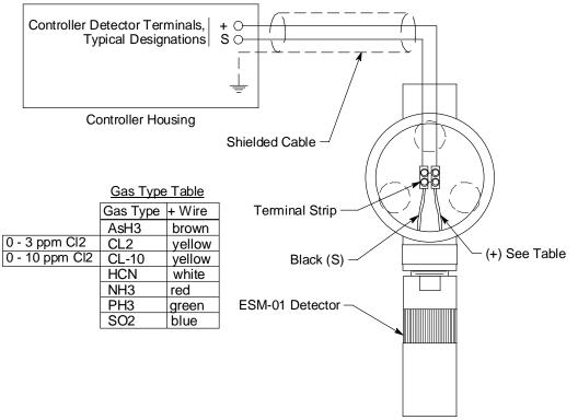
Figure 4: Wiring the Toxic Detector to a Controller
