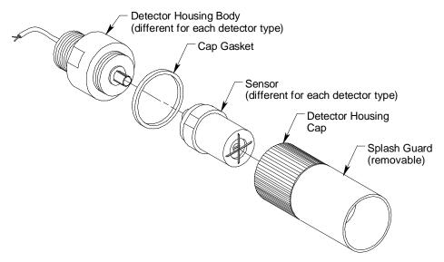
Figure 2: 65-2300RK Toxic Detector Component Location
