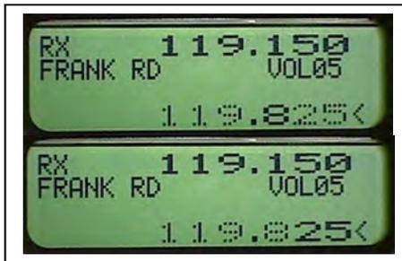
The Standby-Frequency is set with the tuning knob in 3 different ranges. The selected range is highlighted and can be changed with the **FREQ** button.
