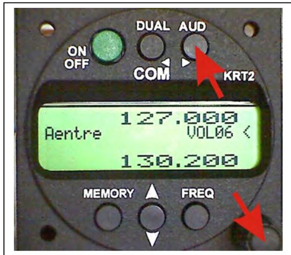
Any action in the Audio Menu requires the pointer (<) to be next to the Audio menu window (see picture). When the pointer is next to the Standby frequency window, the pointer can be repositioned by pressing the AUD button once.
