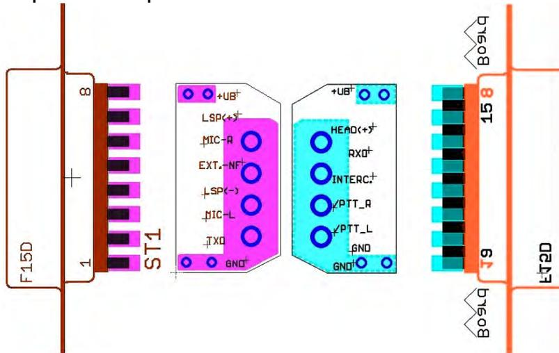
The adapter board is placed between the connector pin rows and soldered to the BAT plus pins 8,15 and GND pins 1,9. Further information printed on the board serves to connect all cables to its corresponding pins.
