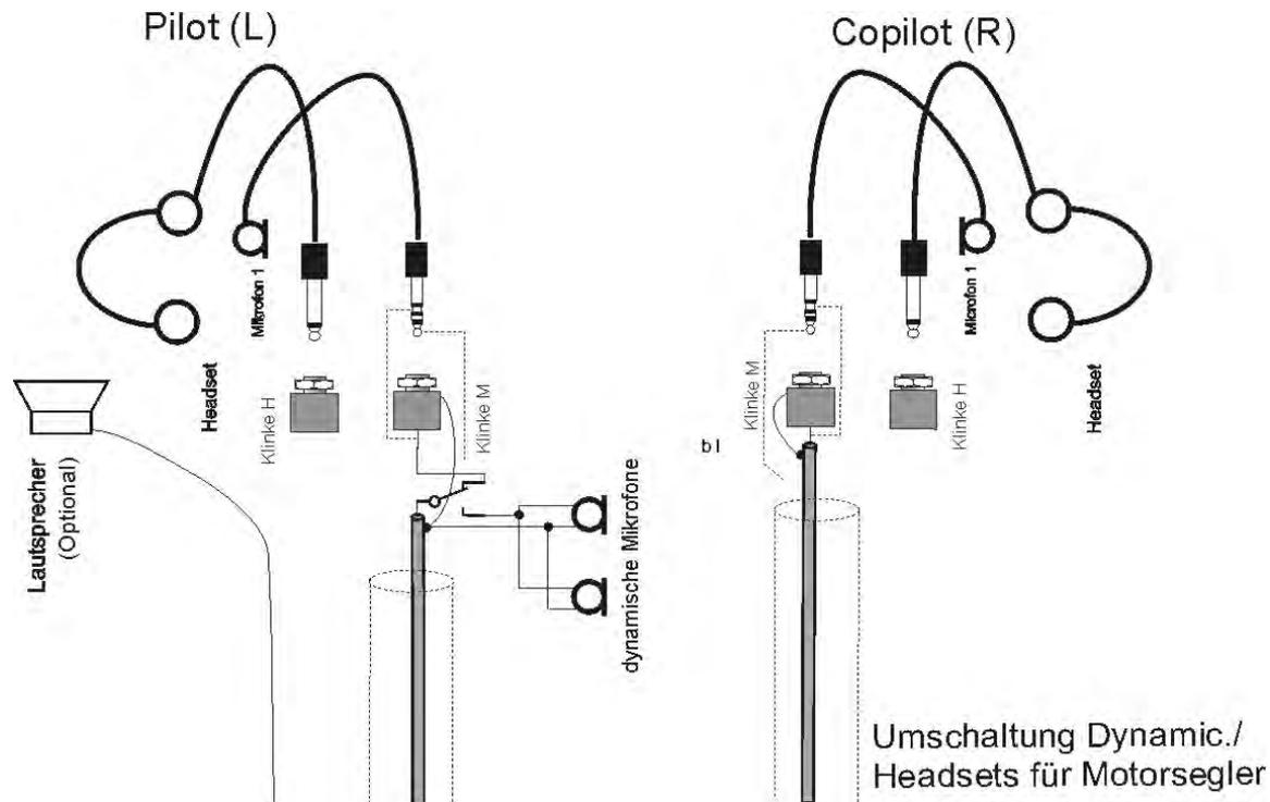
Because the 8V supply voltage is switched off when dynamic microphones are used during glider flight the second (copilot) headset microphone is disabled.
