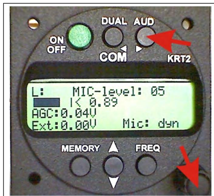
By pressing the DUAL button repeatedly L, R and AUTO can be selected. L (R) means left (right) microphone input channel. The AUTO function is explained later.
