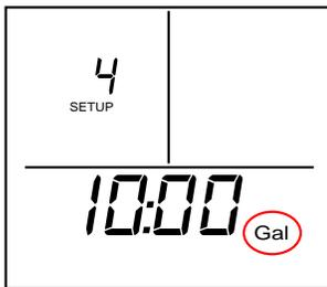
SETUP 4 – Programming the tank/drum/sump capacity (ltr./ Gal.) Enter the number in litres/ gallons then Press **ENTER** to save
