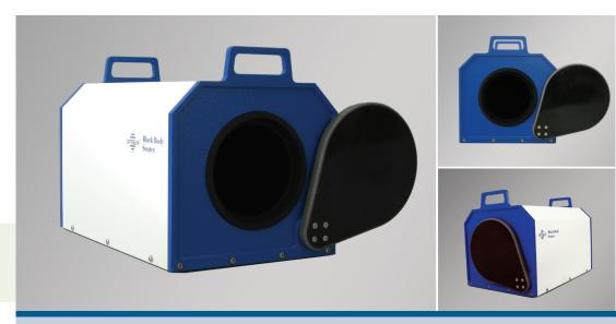
The **BBS-200 Blackbody Source** is a reference source of infrared radiation similar in geometry to the primary standard of the National Physical Laboratory (UK). The blackbody is designed to emit the maximum possible flux at any given temperature. It is used to make a range of important measurements in the 2-14 µm thermal wavebands and is particularly useful for calibrating thermal imagers and radiometers.
