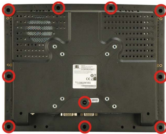
Figure 5-1: Back Cover Retention Screws
