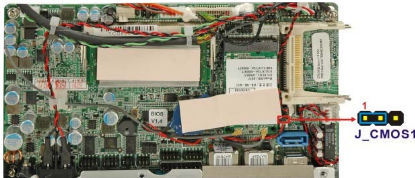
Figure 4-7: Clear CMOS Jumper
