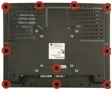
Figure 4-1: Back Cover Retention Screws
