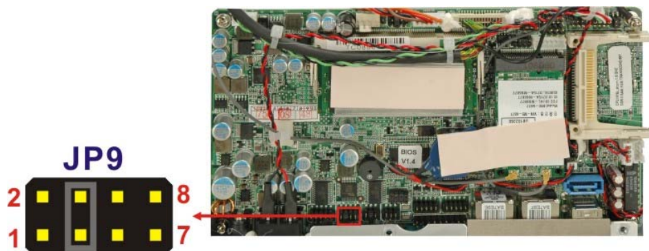
Figure 4-9: COM3 RX Function Select Jumper Location
