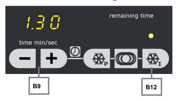
Fig. 26: Setting intermediate cooling
