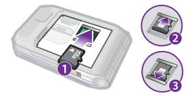
Remove the battery cover and insert the memory card with the gold-coloured contacts facing down.
