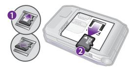
Remove the battery cover and slide the memory card to remove it.
