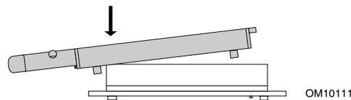
3. Push the lever end of the RM in the direction of the arrow until the two rearmost tabs (D) spread over the end of the AGP universal connector.
