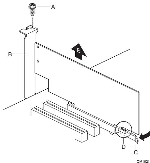
Figure 8. Installing and Removing the AGP Card
