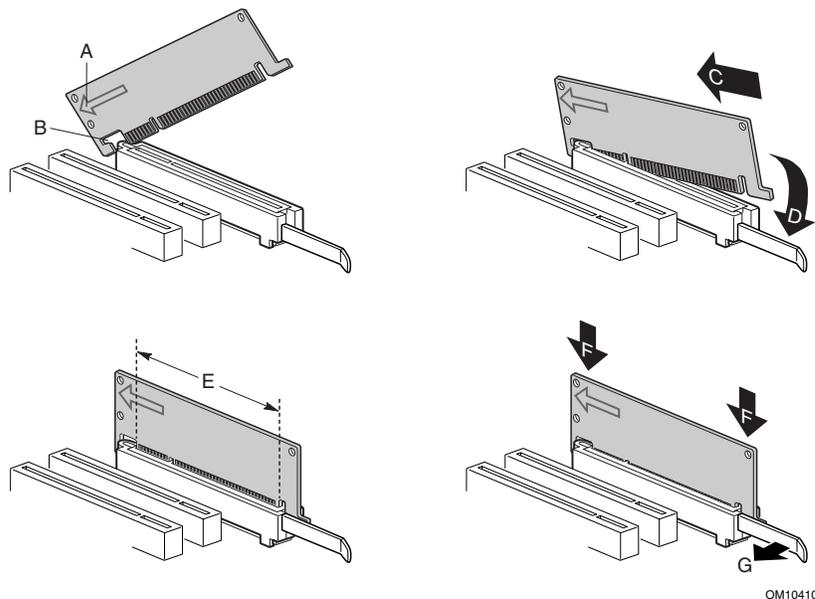
Figure 9. Installing and Removing a GPA Card
