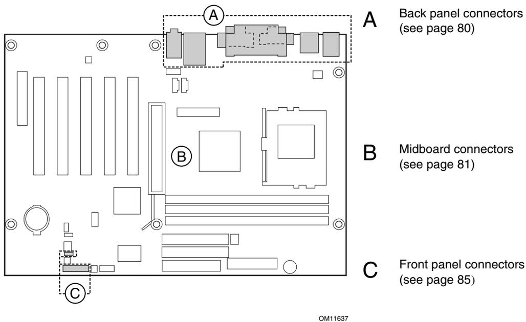
**Figure 27. Connector Groups (the D815EEA2 Board Is Shown)**
