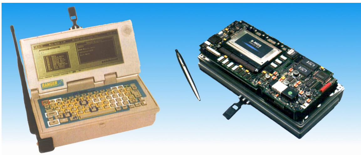
Figure 12-47. Melard "Ranger" Portable Workstation with S-MOS CARDIO Module
