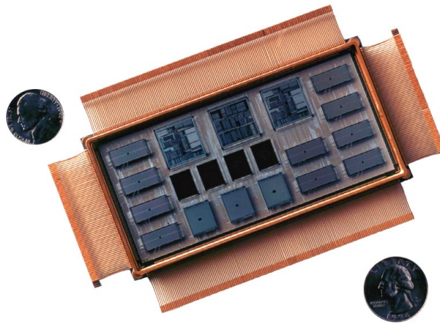
Figure 12-74. Space Flight Computer Module Designed Jointly by TRW and JPL and Built by nCHIP
