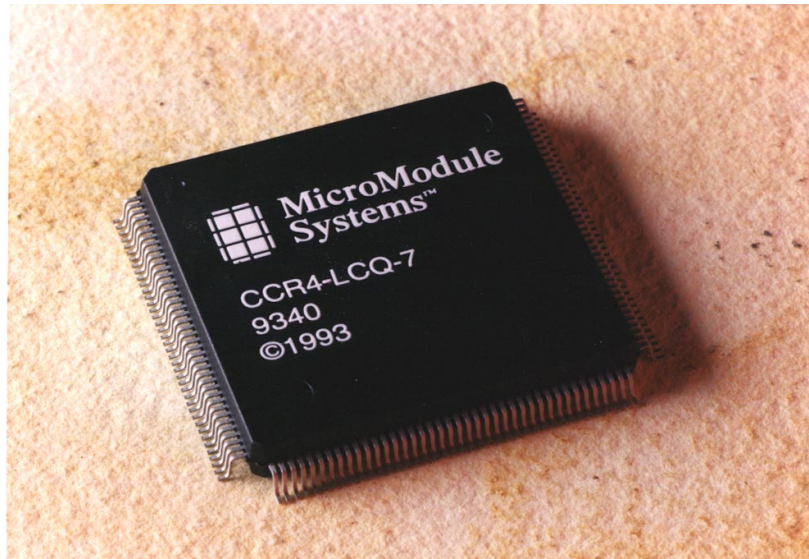
Figure 12-62. ChipFrame Package Consisting of Four SRAM Chips
