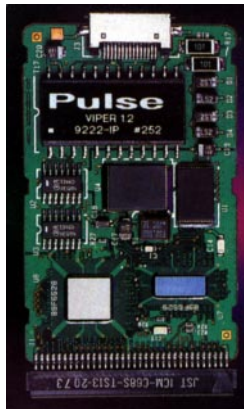
Small Module with Two FC DCA Mounted Chips
