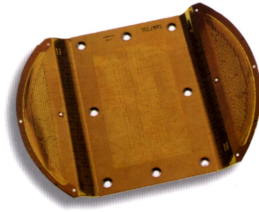
Figure 12-88. Test-Frame Membrane Probe Card for Area Array Chips
