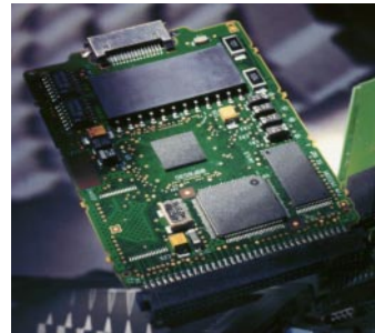
PC-Card with Single DCA Chip
