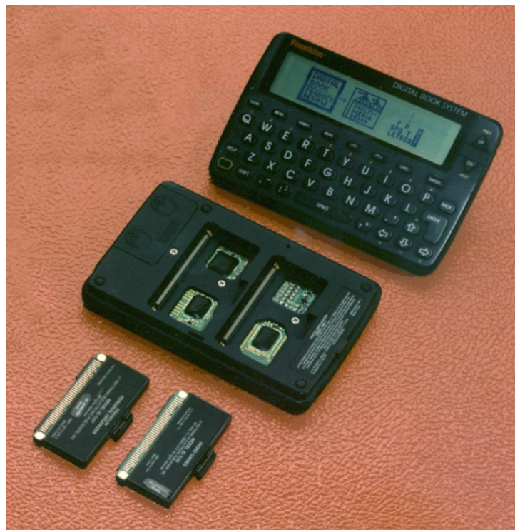
Figure 12-40. Franklin's Handheld Databases with COB Dice
