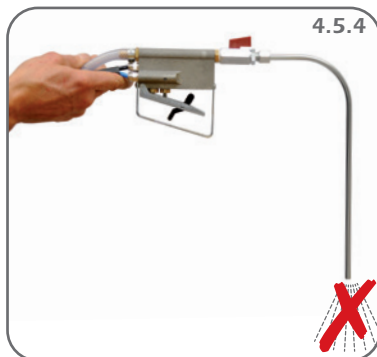
Fig. 4.5.4 No air must come out of the blasting lance unless the hand lever is operated.
