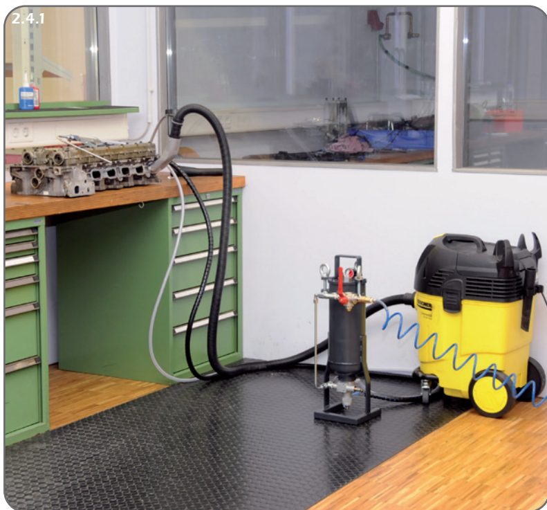
Fig. 2.4.1 The surface on which the device is installed must be level, load-bearing and stable in accordance with the weight of the device.
