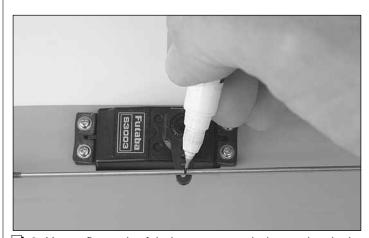
9. Use a fine-point felt-tip pen to mark the pushrod wire where it crosses the outer hole in the servo arm.
