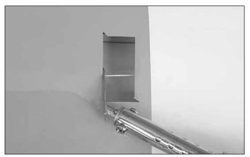
☐ 1. Cut the covering from one (or both) of the aileron servo openings in the bottom of the wings. The "neatest" way is to cut the covering 1/8" [3mm] inside the opening, cut slits up to the corners, and then use a trim iron to seal the edges down inside the openings. Or, just cut the covering up to the edges.
