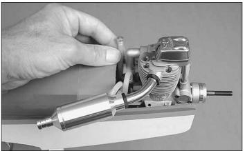
☐ 6. Mount the muffler to your engine and connect the fuel lines to the fuel tank as shown in the diagram. Note that the O.S.® FL .70 has two fuel fittings on the muffler. The fitting with the larger hole goes to the vent line on the fuel tank and the other fitting with the smaller hole goes to the crankcase vent in the backplate of the engine. The line with the fuel line plug goes to either of the "clunk" lines on the fuel tank that will be used for fueling and defueling the tank.
