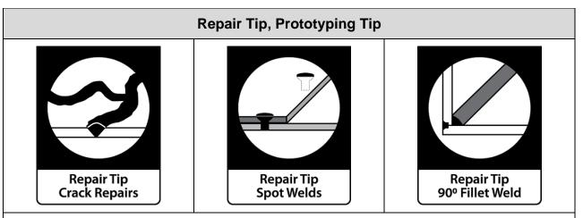
Repair tips are used for crack repairs, filling small holes, spot welding, for reaching tight areas, and for prototyping. Because of their conical shape, the repair tip and prototyping tip offer similar types of welds. Choose the size that best suits your application.
