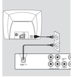
After everything is connected properly, plug in the AC power cord to the power outlet. Never make or change any connections with the power switched on.
