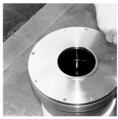
IF FLUID IS LEAKING FROM THE BOTTOM DRAIN REFER TO FLOW RATE INFORMATION IN INSTALL-ATION SECTION AND FOLLOW STEPS TO SET THE FLOW RATE TO THE PROPER VALUE. Periodically inspect this area. It should be clean and dry. DO NOT PIPE OR PLUG THESE HOLES.
