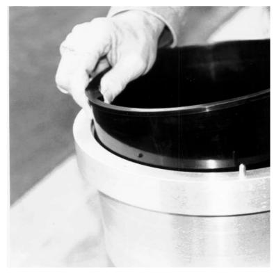
Step Five Discharge the sludge to an appropriate container. Clean the liner to the extent that all of the large material is removed. It is not necessary to wash out the liner to create a scrubbed clean condition. Also clean the vanes on the bottom of the rotor cover removing as much of the sludge as possible.
