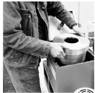
Step Two Set the rotor down on a work surface and, using the hand tool provided, remove the four hex head cap screws securing the rotor cover to the rotor body.
