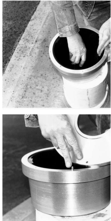
©1996-2013 Bazell Technologies Corporation. All rights reserved. H:\CUSTOMER DOCUMENTATION\Manuals\PDF Manuals\M000012\_A - CF 55 M-2-CE Manual TM.doc. Step Ten Replace the fasteners removed earlier. DO NOT OVER TORQUE FASTENERS. After fully seating the fastener, rotate not more than 1/8 turn. Replace the rotor assembly on the rotor shaft and turn to insure
