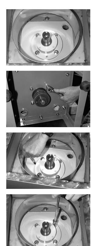
Step 8 Measure and record the distance of the pulley from the bottom of the housing. This will allow you to reset it at the proper height and prevent the misalignment of the drive belts.
