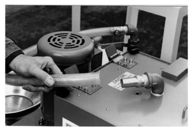
Step Two Place the end of the 1" feed hose over a fivegallon bucket. Open the feed valve and agitation control valve. Using a wristwatch with second hand, note the time to fill the bucket. Set the feed valve to provide approximately 12 GPM.
