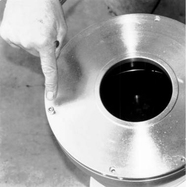
Step Four Remove the rotor liner from the wall of the rotor by pulling inward on the rotor liner and lifting out of the rotor body.
