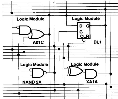
Figure 2. Partial View of TPC10 Series Interconnection Capability
