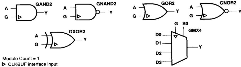
Figure 27. Clock Buffer (CLKBUF) Interface
