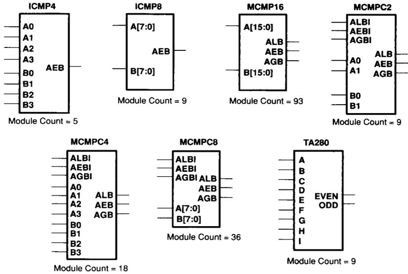
Figure 29. Comparators/Parity Checker
