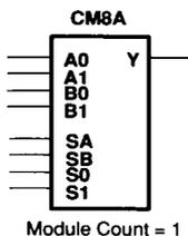
Figure 34. Logic Module
