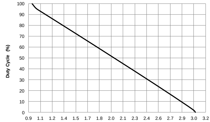
PhLo Output Duty Cycle vs Speed control DC Voltage (SPD)
