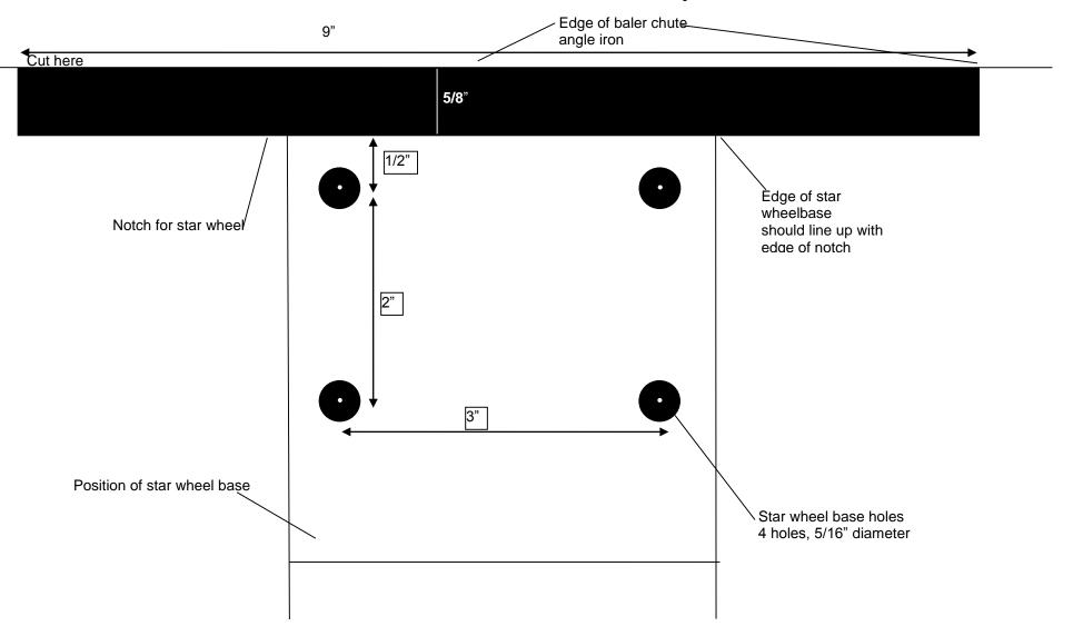
This guide is to be used as a visual aid for star wheel installation. Exact measurements on baler are determined by operator
