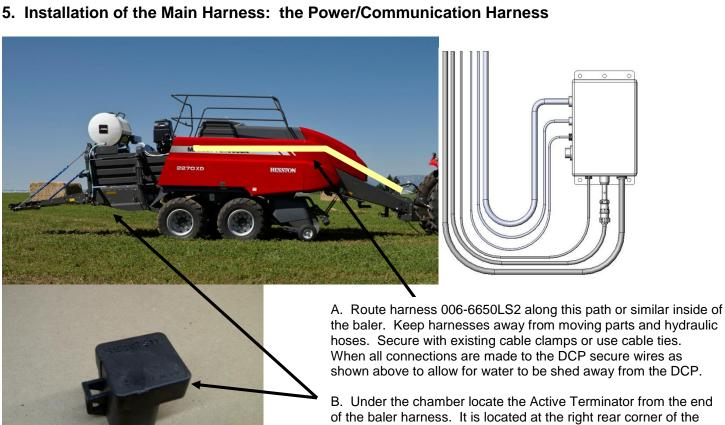
the baler. Keep harnesses away from moving parts and hydraulic hoses. Secure with existing cable clamps or use cable ties. When all connections are made to the DCP secure wires as shown above to allow for water to be shed away from the DCP.
