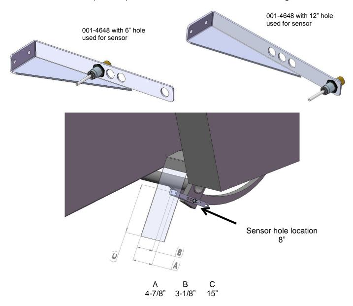
Mount the end of bale sensor bracket (001-4648) as shown. Mark and drill two 5/16" holes and attach the bracket using two 1/4" x 1" bolts, locks, flats, and nuts. Mount the sensor in the 8" hole location, keep the sensor 1/4" from the needle and tighten both nuts. Cut off excess metal past the sensor. Run the sensor cable up to the Dual Channel Processor and secure to the baler.
