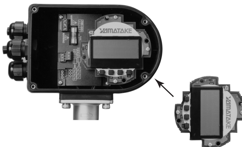
Figure 2-4 Changing the indicator/data setter direction
