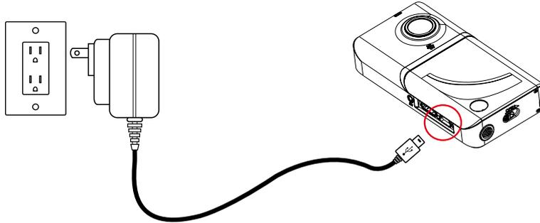
3. When powered on camcorder with power adaptor charging, the battery is in normal charging mode, the charging time is about 5 hours.
