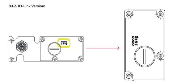
IOL → Flashed green. IO-Link Communications established Lights up permanently green → IO-Link interrupted.
