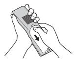
2 Insert the battery (①), and press it down until it snaps into position (②).
