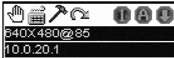
The panel consists of an icon bar at the top, with two text bars below it. Initially, the text bars display the video resolution and IP address of the device at the remote location. As the mouse pointer moves over the icons, the information in the text bars changes to describe the icon's function.
