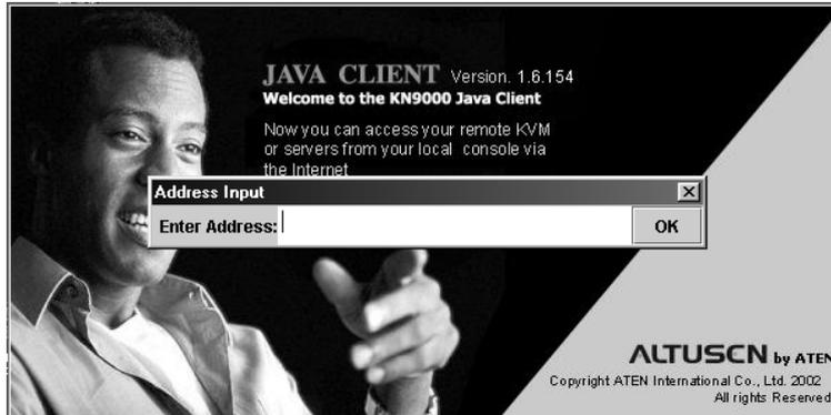
5. Key in the IP address for the unit you want to connect to - including a forward slash followed by the name of the KN9000's Java Client web page.
