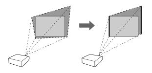
Press ◀ or ▶ to parallelize the upper and lower sides of the projected image.
