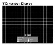
Press ▲, ▼, ◀ or ▶ on the projector or the remote control to adjust the image position.
