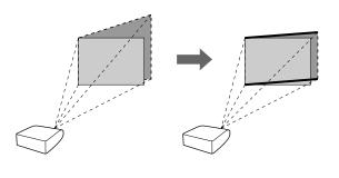
Press on the projector or on the remote control to display "IMAGE RESIZING" and then press ▲, ▼, ◀ or ▶ to correct the image distortion.
