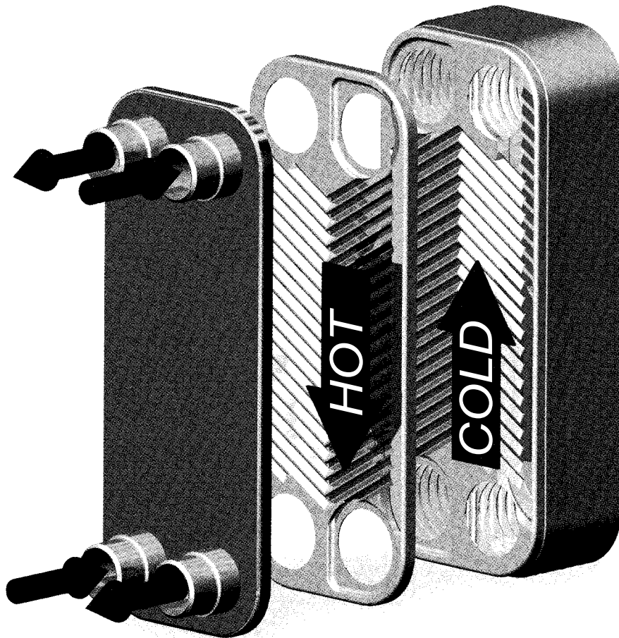
Exploded view of Schmidt SB Braze Plate Heat Exchanger.
