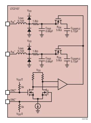
Figure 2. Equivalent Input Circuit
