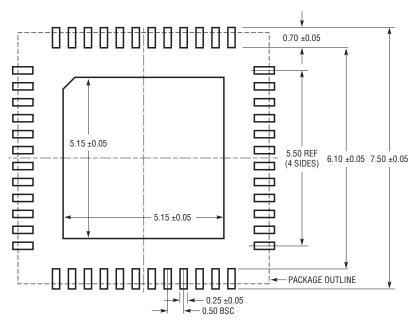
RECOMMENDED SOLDER PAD PITCH AND DIMENSIONS APPLY SOLDER MASK TO AREAS THAT ARE NOT SOLDERED
