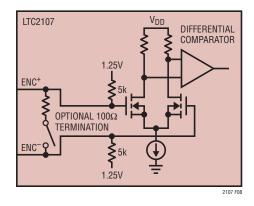
Figure 9. Equivalent Encode Input Circuit
