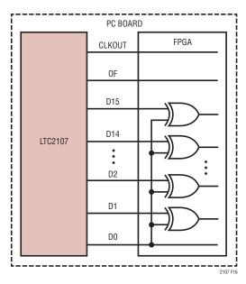
Figure 16. Unrandomizing a Randomized Digital Output Signal
