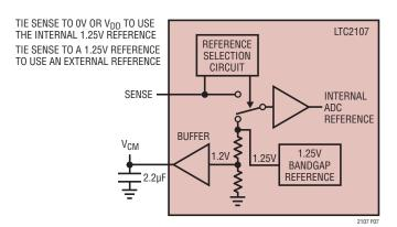
Figure 7. Reference Circuit.
