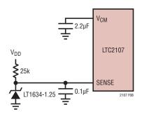
Figure 8. Using an external 1.25V reference.
