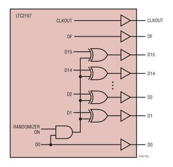
Figure 15. Functional Equivalent of Digital Output Randomizer
