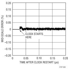
Mid-Scale Settling After Starting Encode Clock with Keep-Alive Off
