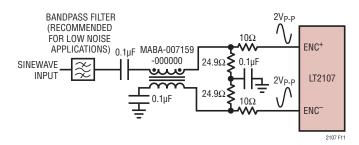
Figure 11. Sinusoidal Encode Drive
