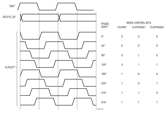
Figure 14. Phase Shifting CLKOUT
