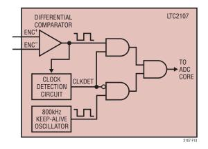
Figure 13. Functionality of Keep-Alive Oscillator
