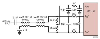
Figure 5. Single-Ended to Differential Conversion Using Two Transformers. Recommended for Input Frequencies from 100MHz to 250MHz
