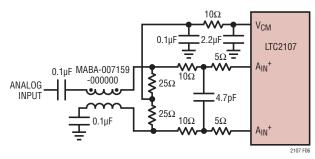
Figure 6. Single-Ended to Differential Conversion Using One Transformer. Recommended for Input Frequencies Above 250MHz
