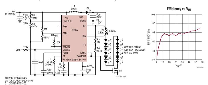
**Boost LED Driver with Output Short-Circuit Protection**
