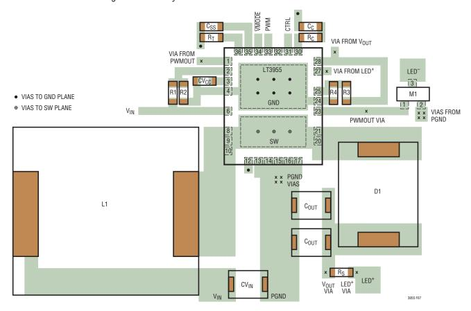
Figure 7. Boost Converter Suggested Layout
