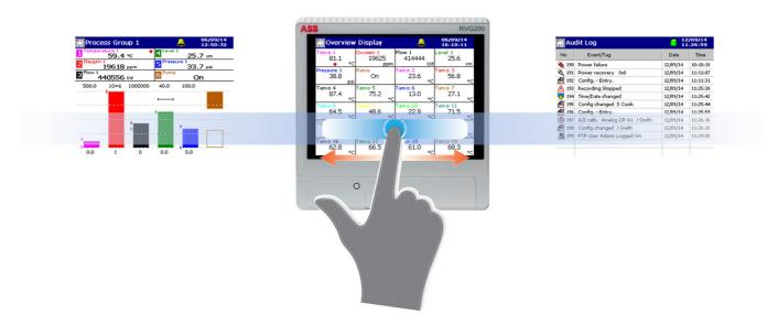
Fig. 2: Navigation using on-screen swipe gestures
