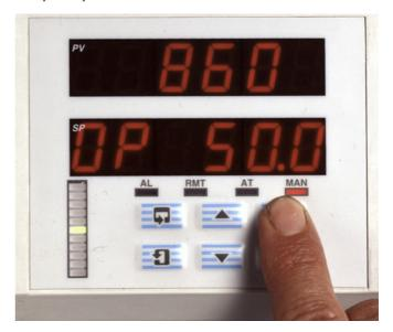
The clearly-labelled tactile keypad gives direct access for operator adjustments and configuration programming, without the need to open the recorder's door. Clear text prompts on the digital displays guide the user around the various menus. A password-protected security system prevents unauthorized access to configuration adjustment menus.
