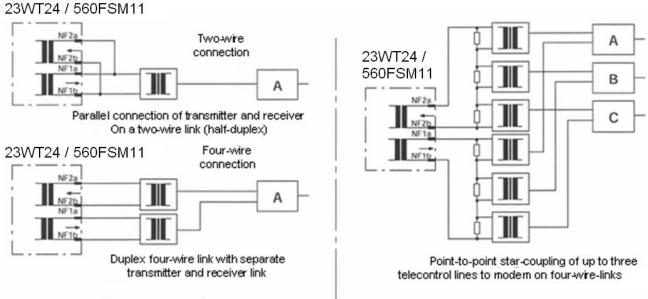
Figure 2: Communication line connection
